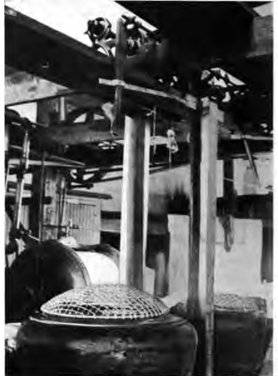
Fig. 2. Extractor with Cover and Latch for Belt Shifter.
